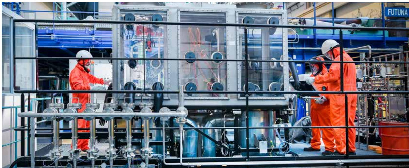
CEA Cadarache – Sodium test loop
